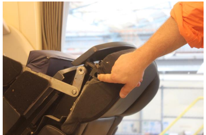
QR staff demonstrate the hinge in the seat mechanism
